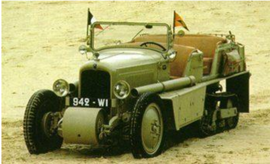
The caterpillar-track Citroen was based on a standard production car that had 1452 cc (developing 20 bhp @ 2 100 rpm) and a 3-speed gearbox driving the twin rear tracks
